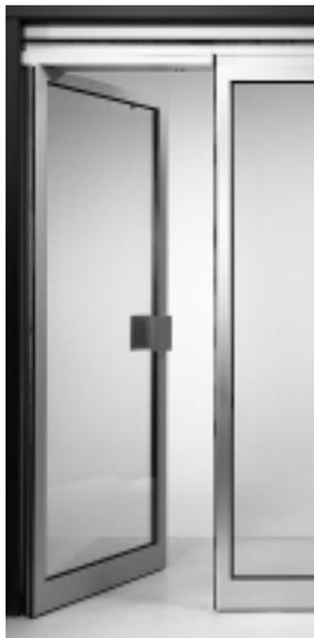
Robust profile frames with top, bottom and side seals for elevated resistance to mechanical loading and protection against weathering, heat loss and draughts. Available with toughened safety glass, laminated safety glass, double glazing or special glazing; standard fixing profile for 8 and 22 mm, other glazing thicknesses on application.
