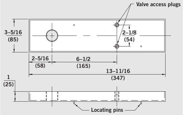
Made from stainless steel and used in lieu of standard floor plate. Offers uninterrupted appearance with terrazzo or marble. Shims are included to allow easy removal of pan after initial installation.
