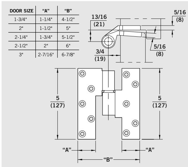
**No. 75240** — 3/4" offset brass intermediate pivot for lead-lined doors 1-3/4" thick.
