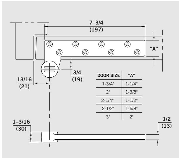
**No. 75343** — 3/4" offset steel bottom arm for lead-lined 1-3/4" doors.
