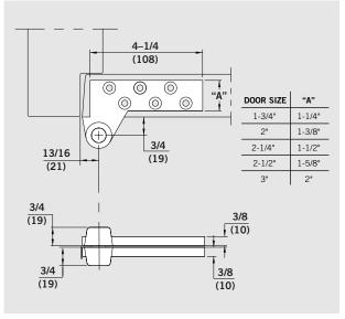
**No. 75140** — 3/4" offset brass top pivot for lead-lined doors 1-3/4" thick.
