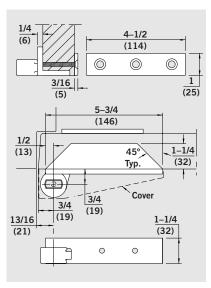
$\begin{tabular}{ll} \textbf{No. 75353} & -3/4" offset steel bottom arm. Closer is removable without removing door. Intermediate pivots are required when using this arm. \\ \end{tabular}$
