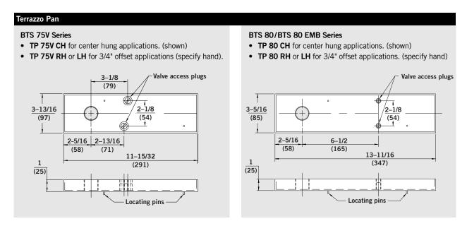
Made from stainless steel and used in lieu of standard floor plate. Offers uninterrupted appearance with terrazzo or marble. Shims are included to allow easy removal of pan after initial installation.
