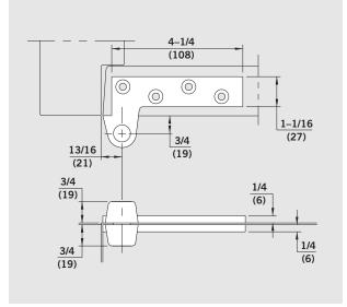
No. 75120 — 3/4" offset brass top pivot. No. 75122 — 3/4" offset brass top pivot. U.L. listed for 20-minute rated fire doors. No. 75133 — 3/4" offset steel top pivot. For use on fire doors rated up to three hours.
