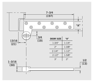
**No. 75343** — 3/4" offset steel bottom arm for lead-lined 1-3/4" doors.
