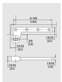
**No. 75323** — 3/4" offset standard-duty steel bottom arm. Can also be used on fire doors rated up to three hours.
